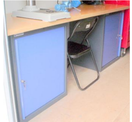
Dual Pedestal Workbench, 40 mm thick wood top, Dimensions; 2000 mm W x 840 mm H x 600 mm D
